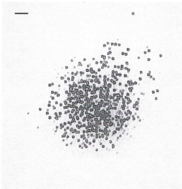
**Figure 2. A typical group of etch pits here called a cluster. It is a high-density grouping of pits without any orientational arrangement among them, occupying an area of the detector chip otherwise fairly devoid of etch pits. (Scale line = 82  $\mu\text{m}$ ).**
