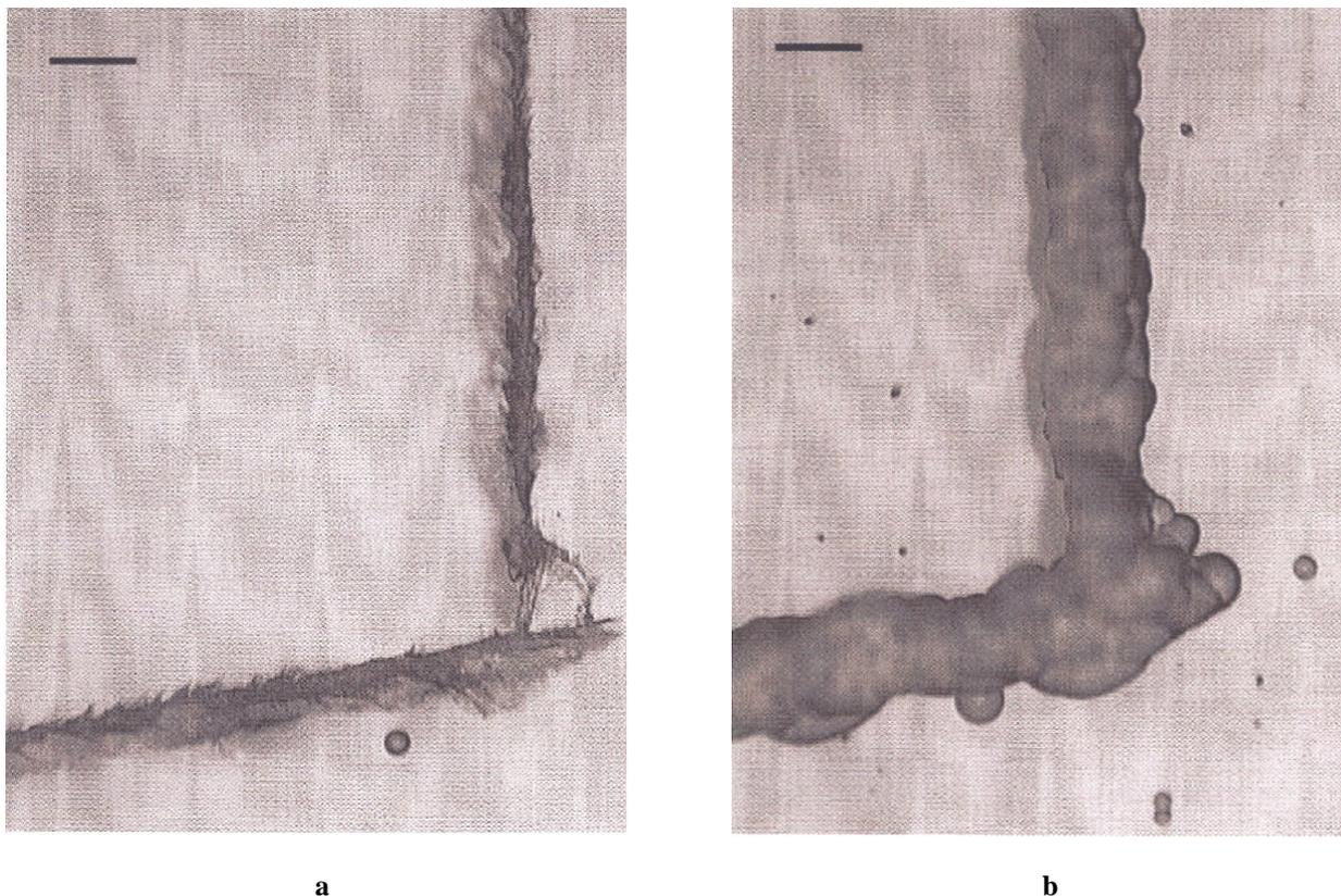
**Figure 5a. Photomicrograph (Scale line= 80  $\mu\text{m}$ ) of a region of a CR39 chip after the first etch. The L-shaped figure was scratched after the first etch in order to be able to locate the same region after re-etching. Only one pit appeared after the first etch. 5b. Photograph of the same region after the second etch. The scratch mark has thickened and almost covers the original single pit, and a new family of pits has appeared, produced by the second etch.**
